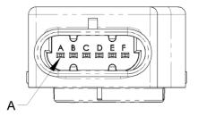
Mating connector type: Packard Electric 'Metri-Pack' 150 series or equivalent Mating Part Nos: 12066317 (housing) & 402418 (terminal, female)
