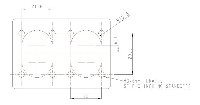
Curtiss-Wright recommend that the JC040 rocker is mounted using a minimum of two M3 x 6mm female, self-clinching standoffs (e.g. PEM ref. CSS M3-6) fitted to the back of the panel at diametrically opposite positions. The standoffs are used in conjunction with two M3 x 6mm washer head screws. The screws should be tightened to a torque of 0.4Nm to 0.7Nm with a minimum panel thickness of 3 mm.
