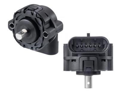
The WM-H10 shaft-operated Rotary Position Sensor is a solid-state, Hall-effect sensor offering two independent and electrically isolated outputs in a compact housing with integrated connector.
