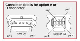
When connecting the sensor, care should be taken with the correct connections. The sensor is provided with indefinite reverse polarity protection and short circuit protection between output to GND (Black), but if the outputs are connected to the supply this will result in device failure.
