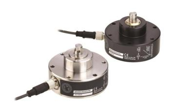
The SRH880P sensor operates from 9-30Vdc unregulated or 5Vdc regulated supply and is available with analog (0.5-4.5Vdc) or digital (PWM) output signals. The sensor is factory programmable, allowing you to specify the output signal type, the measurement range (0-20° to 0-360° in 1° increments) and the output direction (clockwise or anticlockwise).
