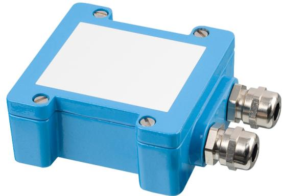
The UCM is a low powered Universal Conditioning Module designed to operate with a wide range of LVDTs, RVDTs and other analogue inductive transducer types. The set-up is simple and flexible, allowing user adjustment of excitation voltage and frequency, operating mode, span output and zero position, as well as configuration for multiple unit synchronisation
