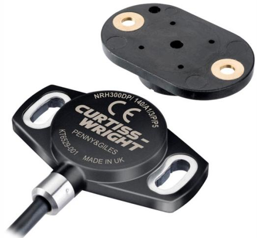
The NRH300DP is a no-contact, Rotary Position Sensor that offers the optimal combination of performance, safety and cost. The sensor utilises proven Hall-effect, sensing technology in a low-profile (8mm) housing with separate magnet for true no-contact sensing.
