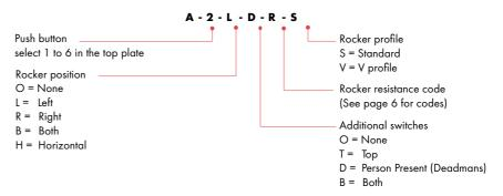
Note: When ordering a handle fitted with a rocker, two profiles can be supplied (S = standard profile; V = v profile) please specify style when ordering.
