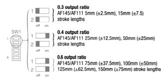
Step 4 Set output span using switches 3 and 4 on SW1 as shown
